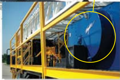
The heavy-duty mechanical drawworks with disc brakes provides 37,500 lbs. of single line pull, and the simple yet powerful state-of-the-art brake system includes redundant safety systems including crown and floor savers.
