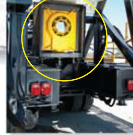
The hydraulic rotary table provides up to 60 inches of vertical conductor clearance and hydraulically lifts out of position to allow for a full 42 inches of casing clearance through the frame.
