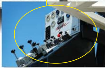
The operators console provides excellent visibility and a simple user-friendly control layout. Controls for all drilling functions, including weight indicator, crown and floor savers are all easily accessible from the console.
